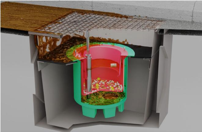
Liquids are retained when the isolation valve is in the closed position.
